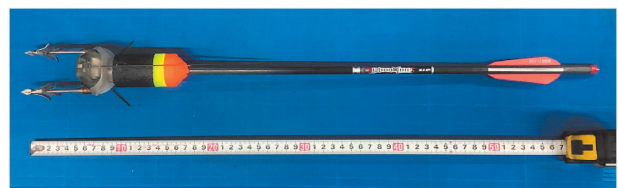
Figure 8. A set of SPLASH10-F-333 and its carrier are designed for a crossbow manufactured by Wildlife Computers.
