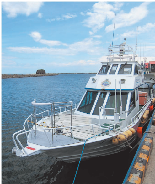
Figure 2. Whale-watching boat "Chipashiri" (4.9t; 10.45 m). A safety fence was installed at the bow during the survey. The height of bow deck is 130cm from the water.
