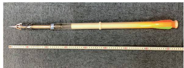
Figure 2. SPOT6-type tags (Wildlife Computers Inc.) connected to ICR's ISOD-type anchor and LK-Carrier.
