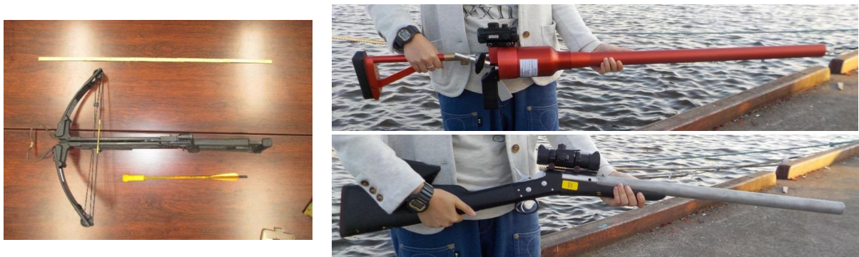
Fig. 2. The equipment for biopsy sampling. Compound crossbow (left); air gun (LKARTS-Norway; right upper); Larsen gun (right lower).
