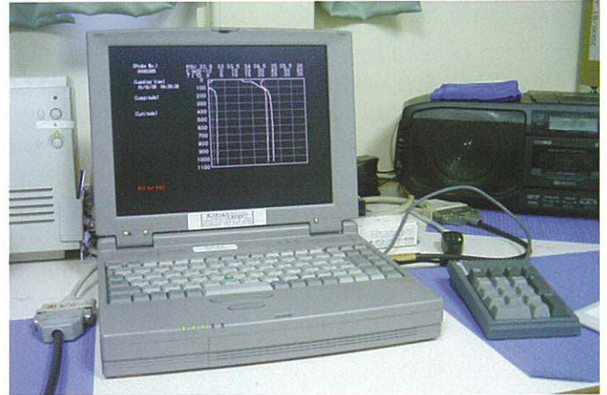
Fig. 22. XCTD data monitor. Oceanographic survey data are processed on board.
