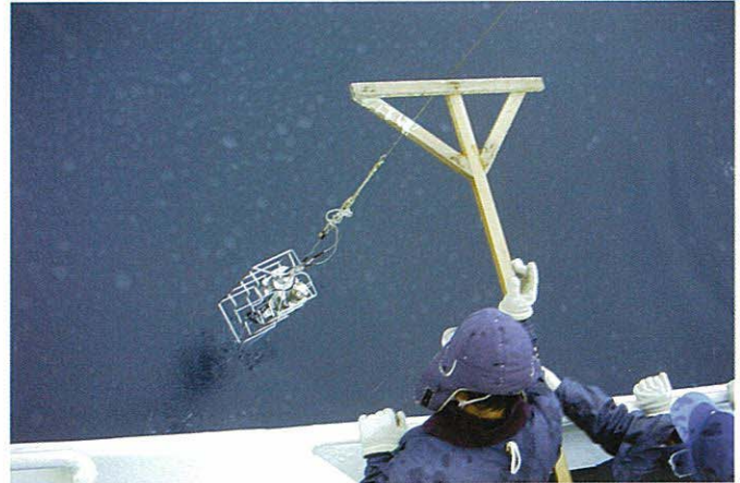
Fig. 76. CTD observations. The CTD is thrown into the sea to collect data on the vertical profile of water Conductivity (salinity), Temperature, and water pressure (Depth).
