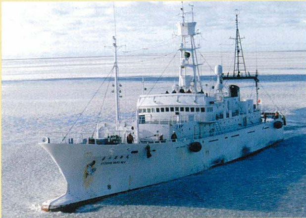
Fig. 13. The dedicated sighting vessel Kyoshin Maru No. 2 navigating ice floes in the Antarctic Ocean. Conducts echo-sound research on krill resources and oceanographic surveys besides sighting surveys (68.18 m, 372 tons).
