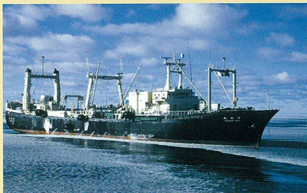
Fig. 17. The research mothership Nisshin Maru. From here instructions are given to the sighting/sampling vessels. Biological surveys and processing of by-products are performed here (129.58m, 7,659 tons).
